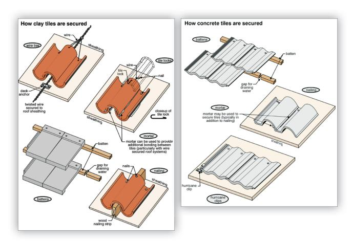
WEAR FACTORS Like any brittle roofing system, concrete and clay tiles are subject to mechanical damage, and like any long-lasting roof system, the fasteners may wear out before the tiles. Depending upon the design of the roof system, they can be very difficult to repair.
